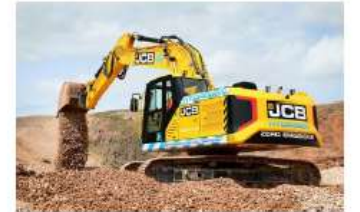
JCB hydrogen excavator
