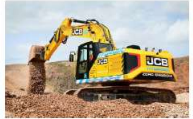
JCB hydrogen excavator
